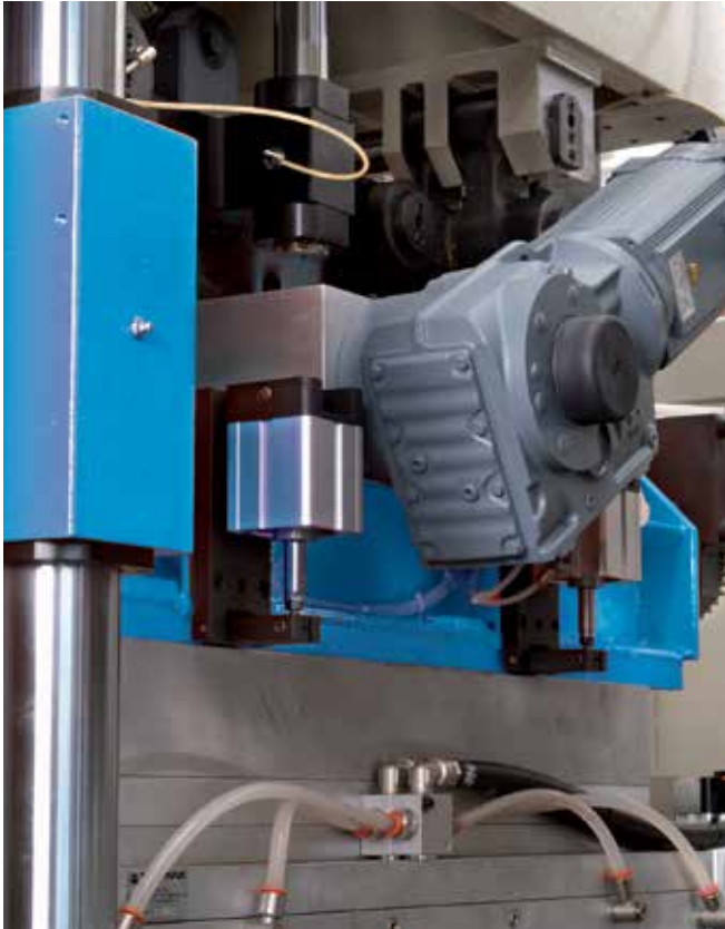
Servo-motor driven plug assembly
