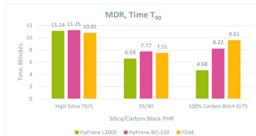
Figure 3: Comparison of T 90 cure time for the three process oils with different filler loadings
