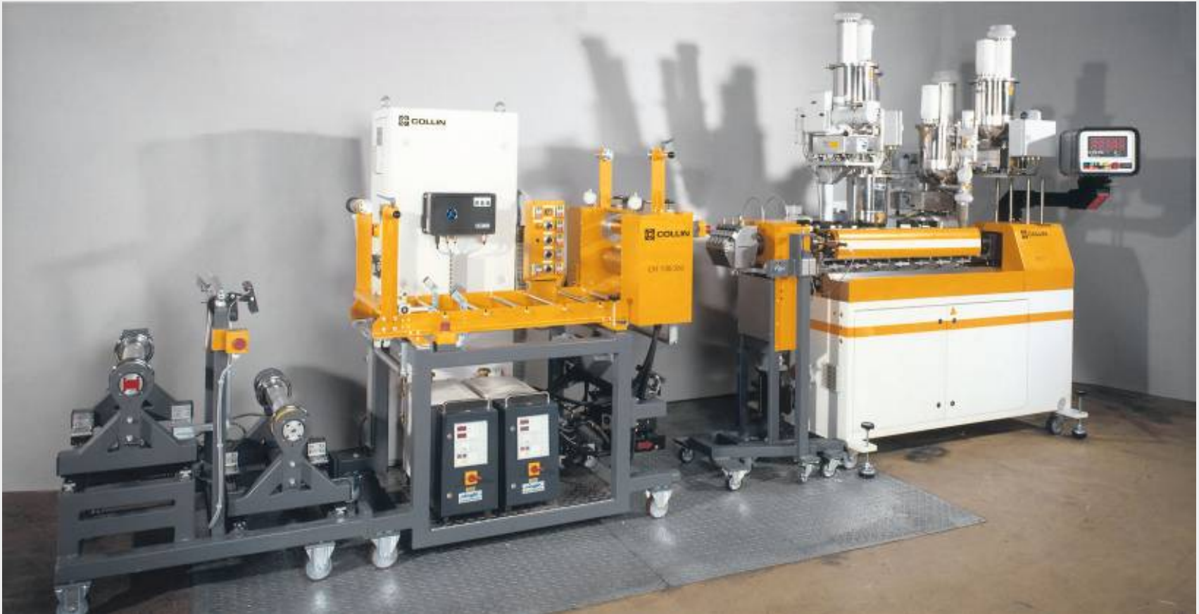
Kneader Type ZK 25 with 4x Feeding, Melt Pump, Die and Finishing Unit for Sheets
